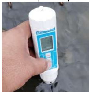
Image 6-8: Takiya Ghat Phytoremediation Project DO of 1.3 at Starting Point (left) and DO of 2.9 at outlet of River Rapti (right)
