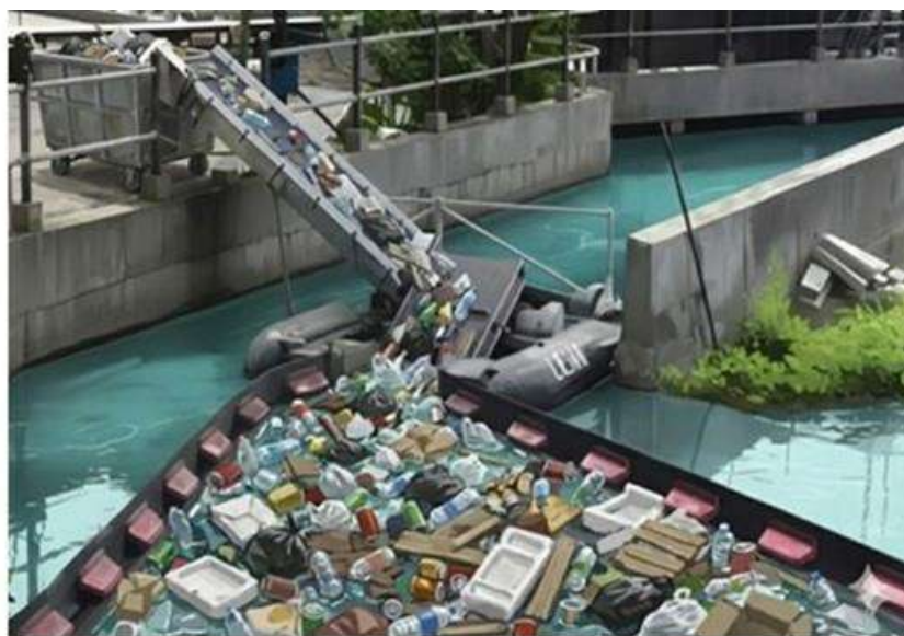
Figure 6-3: Conceptual arrangement of proposed Litter Trap
