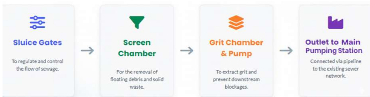
Figure 6-1: Flow arrangement of proposed I&D Structure
