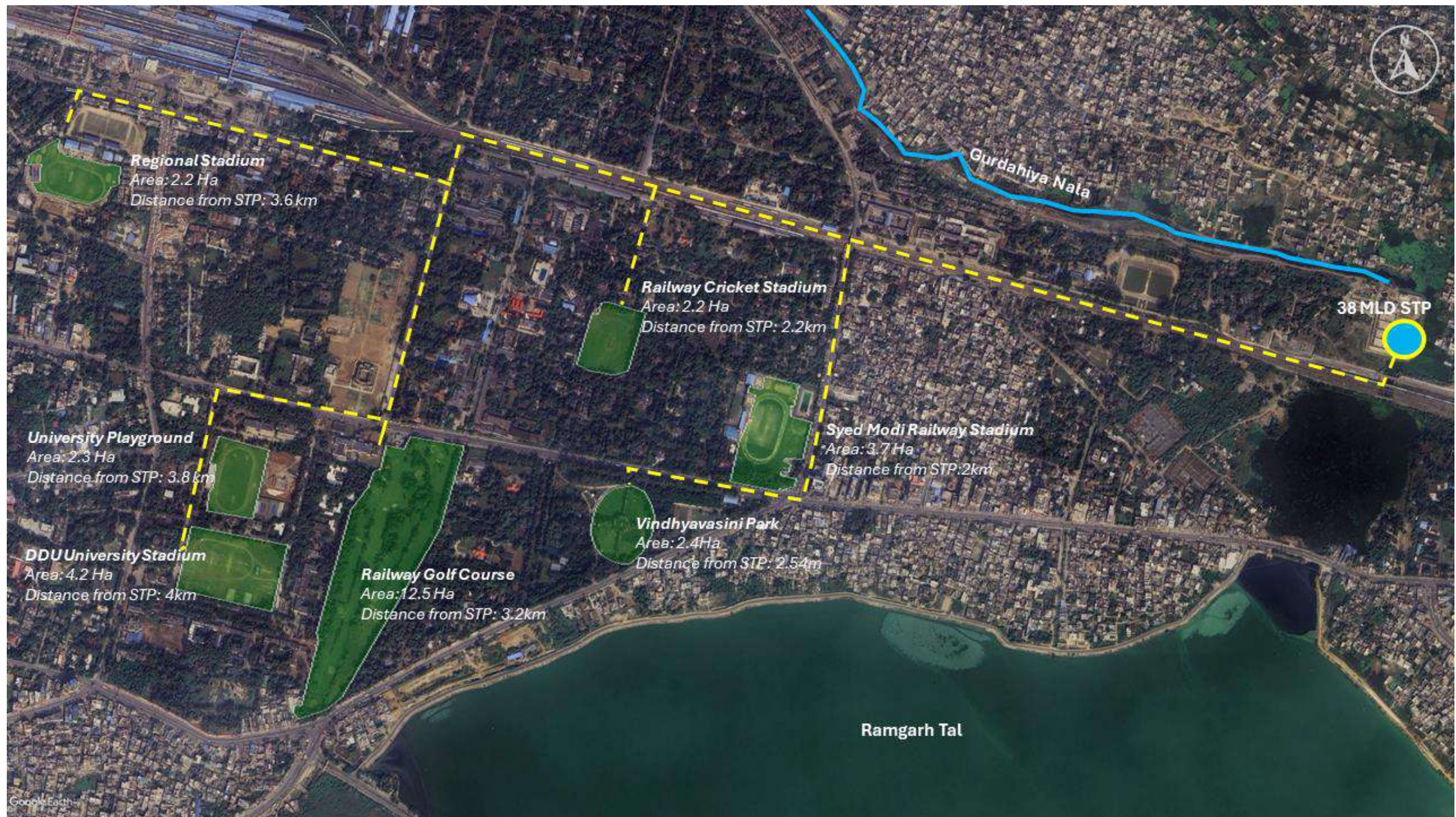
Map 6-5: Proposed reuse of treated used water from 38 MLD STP in various organized greens in close proximity
